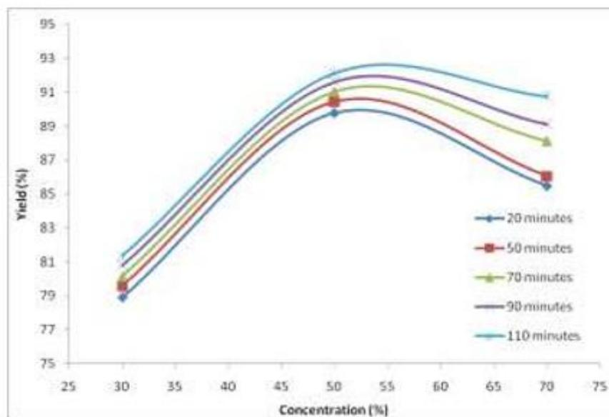
Figure 2. Chart effect relationship sulfuric acid concentration vs time at stirring speed of 200 rpm, 190 °C and sulfuric acid and kaolin ratio of 3: 1
